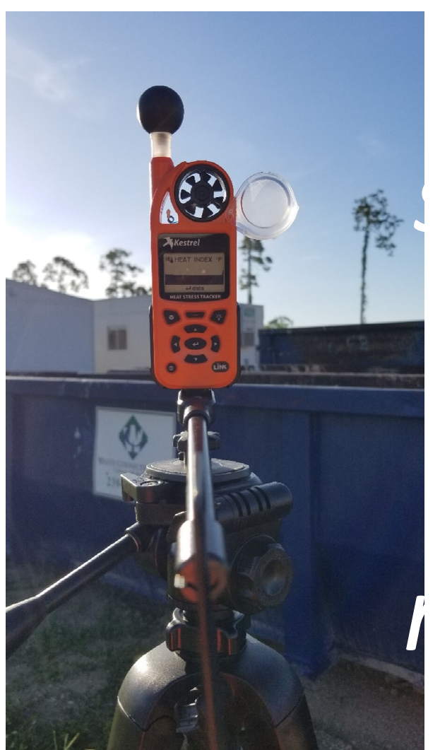
Fig. 1. Kestrel 5400 Heat Stress Tracker Setup
