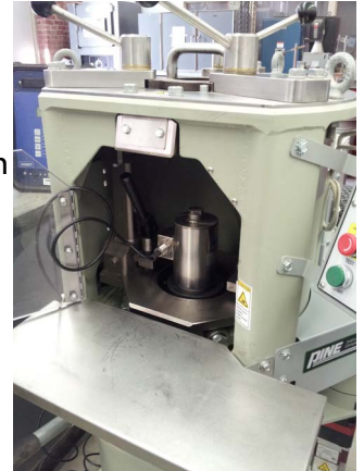
Calibration of CP 2 Center's superpave gyratory compactor
