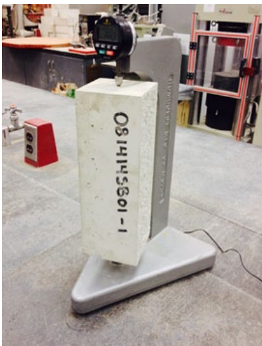
Figure 5. Shrinkage measurement on a prism sample by us- ing a length comparator, which mea- sures speci- men length change
