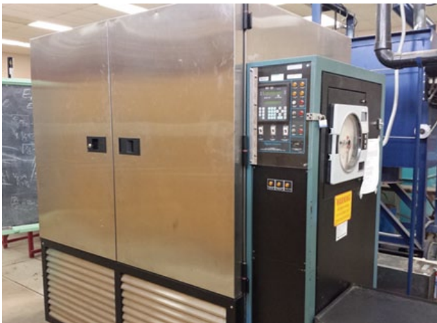
Figure 4. Concrete en- vironmental chamber for drying concrete samples
