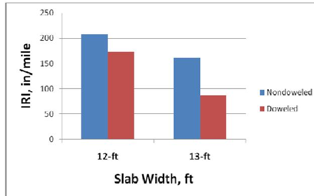
**Figure 7. Impact of concrete overlay slab width on doweled and nondoweled IRI (for 8-in. JPCP) using the MEPDG.**
