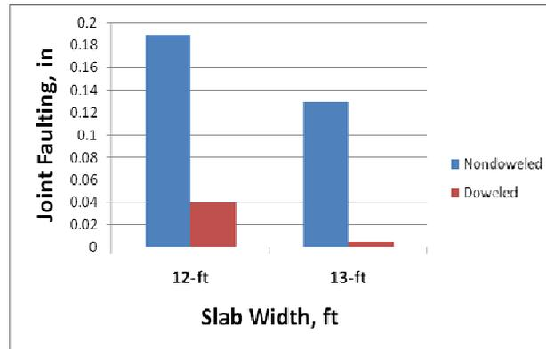
**Figure 6. Impact of concrete overlay slab width on doweled and nondoweled joint faulting (for 8-in. JPCP) using the MEPDG.**
