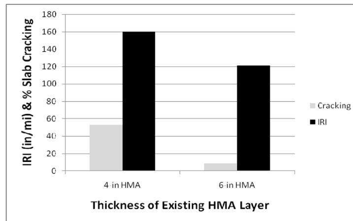
**Figure 4. Effect of “Poor” HMA layer thickness on IRI and transverse cracking of the JPCP overlay.**
