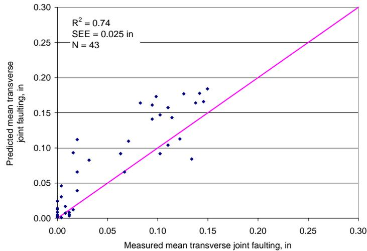
**Figure 2. National calibration plot for joint faulting of unbonded JPCP overlays.**
