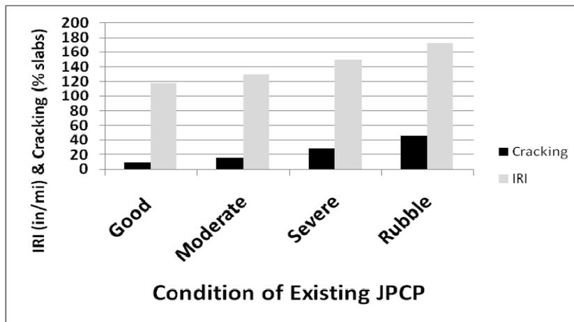
**Figure 8. Effect of condition of existing JPCP on IRI and transverse cracking of JPCP overlay after 30 years and 55 million trucks (93 million ESALs).**
