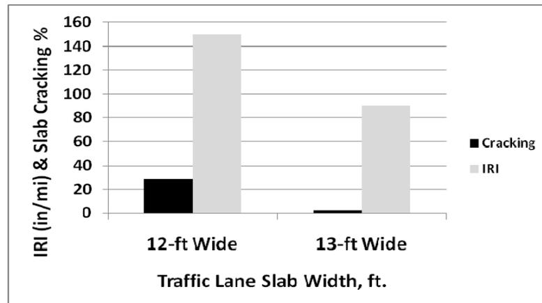
**Figure 10. Effect of traffic lane slab width on slab cracking and IRI after 30 years and 55 million trucks.**
