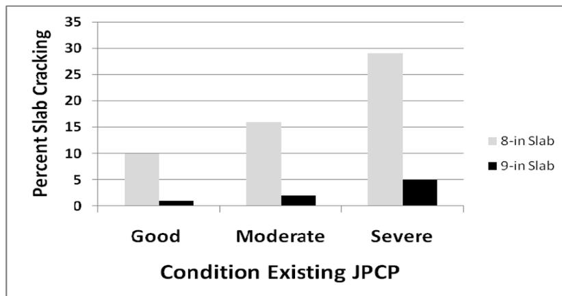
**Figure 9. Effects of condition of existing JPCP and slab thickness on percentage of slab cracking after 30 years and 55 million trucks.**
