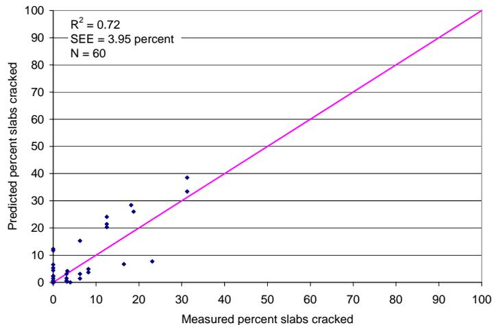
**Figure 1. National calibration plot for transverse cracking of unbonded JPCP overlays.**
