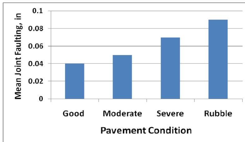
**Figure 11. Effect of existing JPCP condition on transverse mean joint faulting after 30 years and 55 million trucks.**
