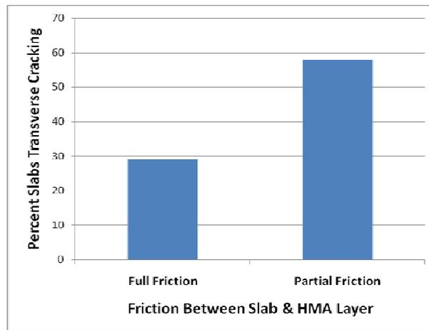
**Figure 5. Effect of Slab/HMA friction on slab cracking (partial means no friction after 60 months).**
