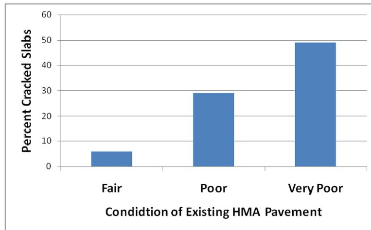
**Figure 3. Effect of condition of existing 4-in. (102-mm) HMA pavement alligator cracking on 6.5-in. (165-mm) JPCP concrete overlay slab cracking after 30 years and 8.4 million truck loadings (14 million ESALs).**
