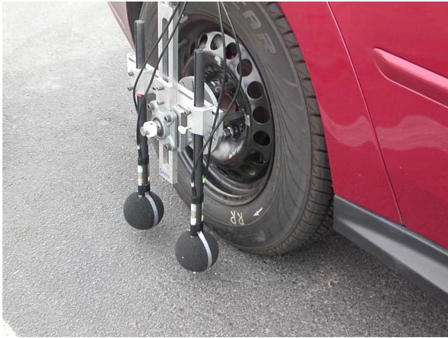
**Figure 3. OBSI microphone setup—two-probe system.**
