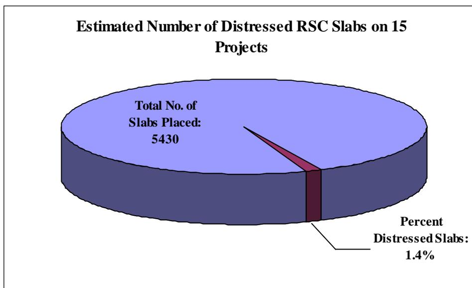
**Figure 9. Percent distressed slabs on surveyed RSC projects (13).**
