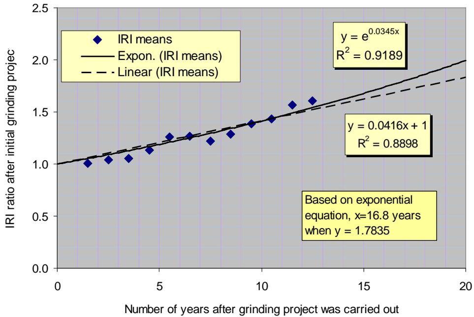
**Figure 1. Change in the ratio of IRI over time as a function of the initial IRI after grinding (2).**
