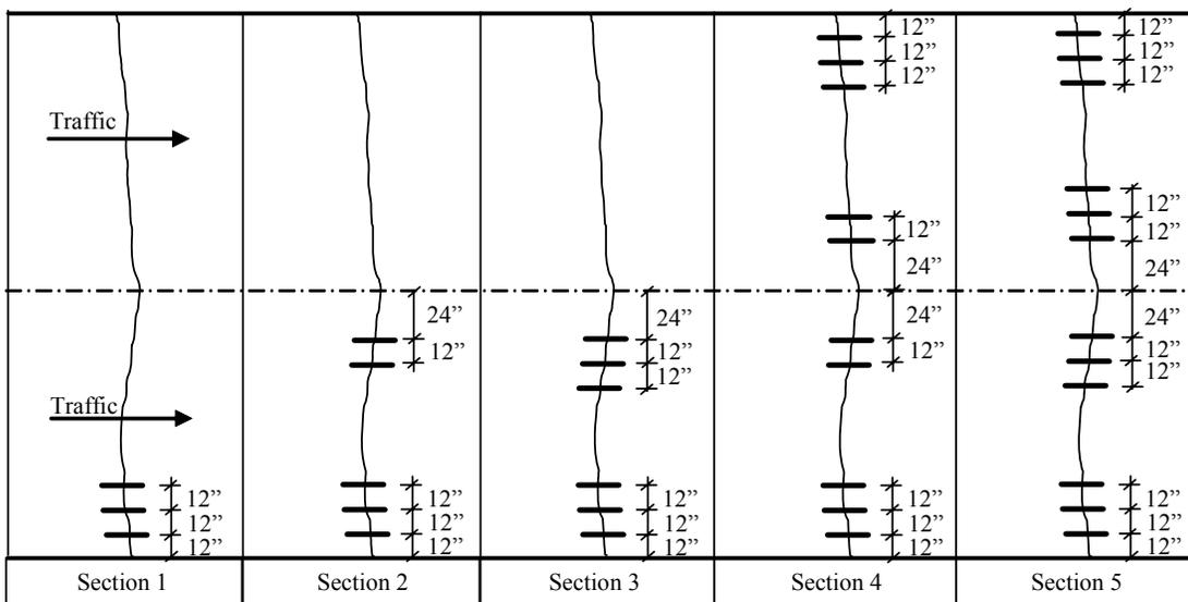
Figure 1. TH 52 test section retrofit dowel bar patterns.
