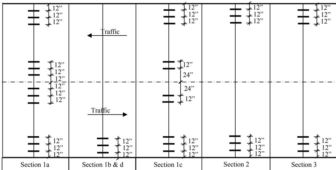
**Figure 3. TH 23 test section retrofit dowel bar patterns.**
