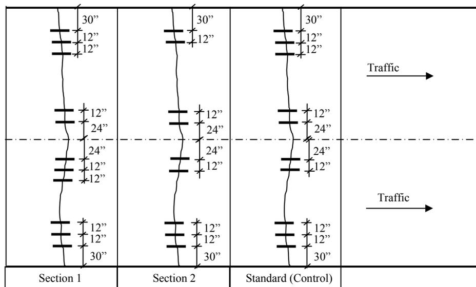
**Figure 4. I-90 Test section retrofit dowel bar patterns.**
