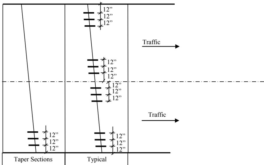
**Figure 2. TH 12 test section retrofit dowel bar patterns.**
