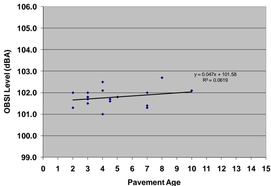
Figure 14. Acoustic durability of conventional diamond-ground projects in Kansas.
