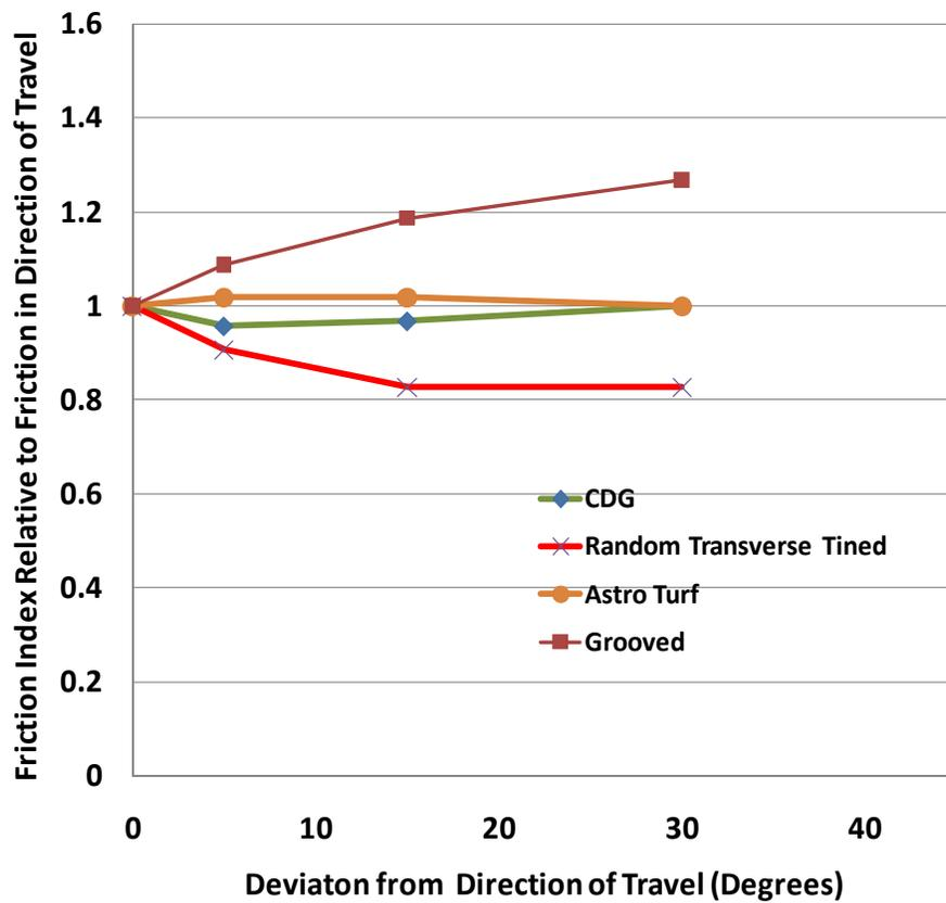
Figure 16. Friction index as a function of deviation from the direction of travel (uncorrected for cross slope).
