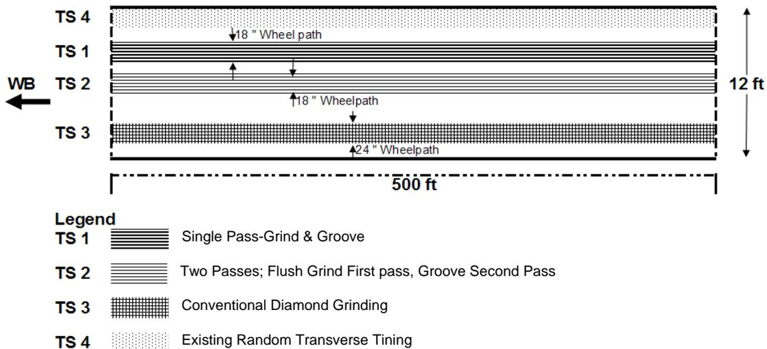
**Figure 5. Proof of concept field test strips at MnROADS low-volume roads test area.**
