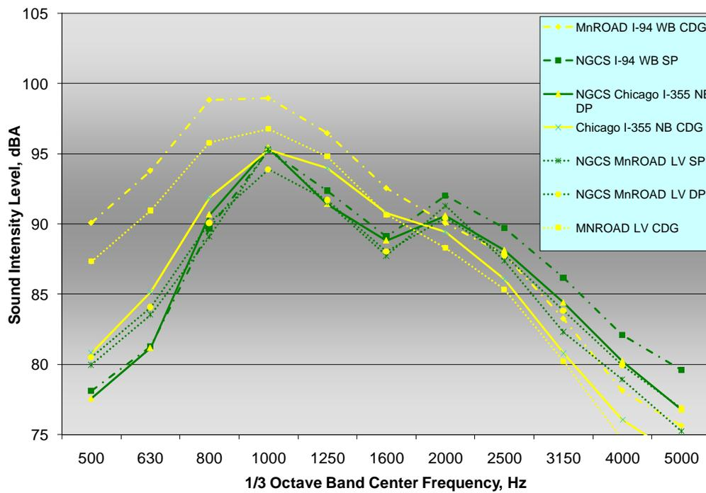
Figure 7. One-third octave spectral plots for MN I-94 and IL I-355 sections.
