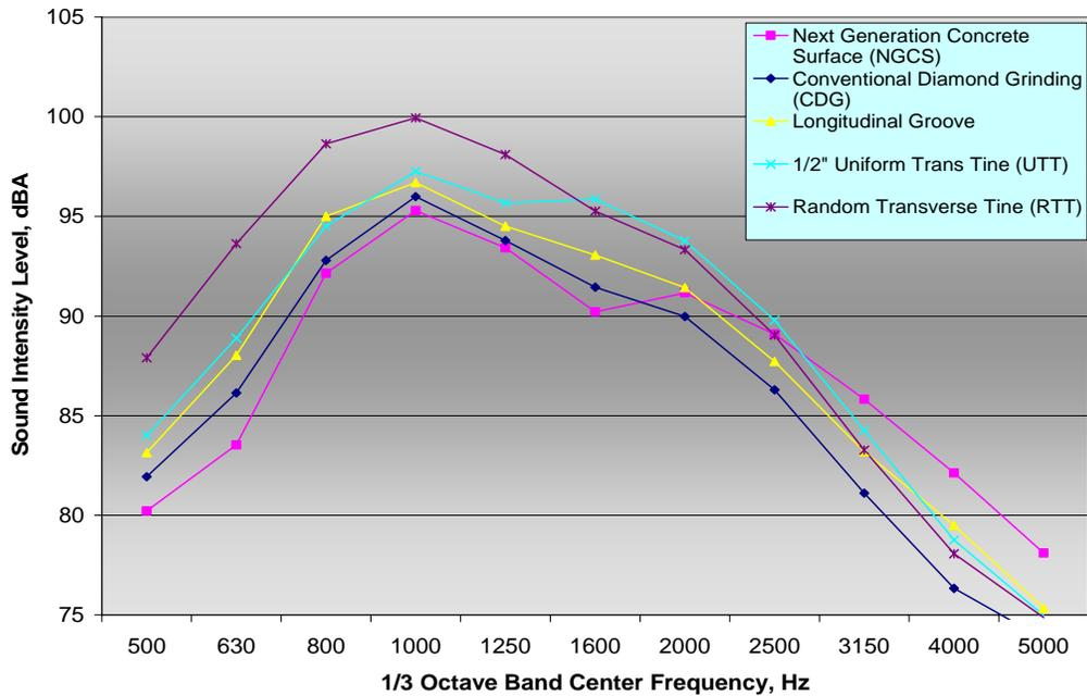
Figure 9. Chicago I-355 OBSI spectrum results of selected textures tested November 4, 2007.
