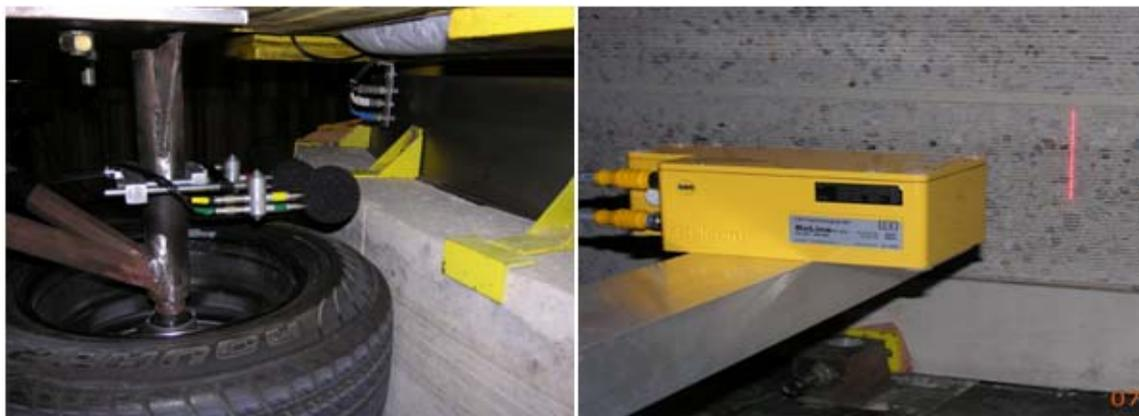
Figure 2. OBSI and RoLine test equipment mounted to TPTA.
