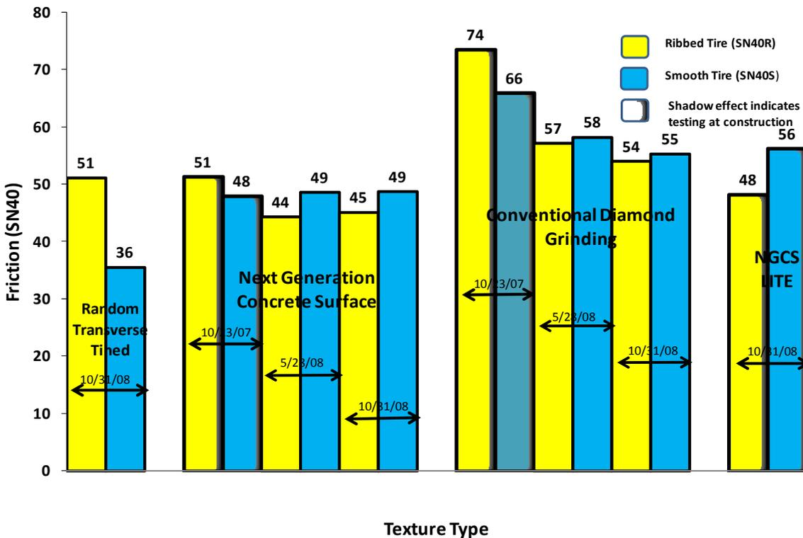
Figure 13. Friction (SN40) as a function of surface texture and time.
