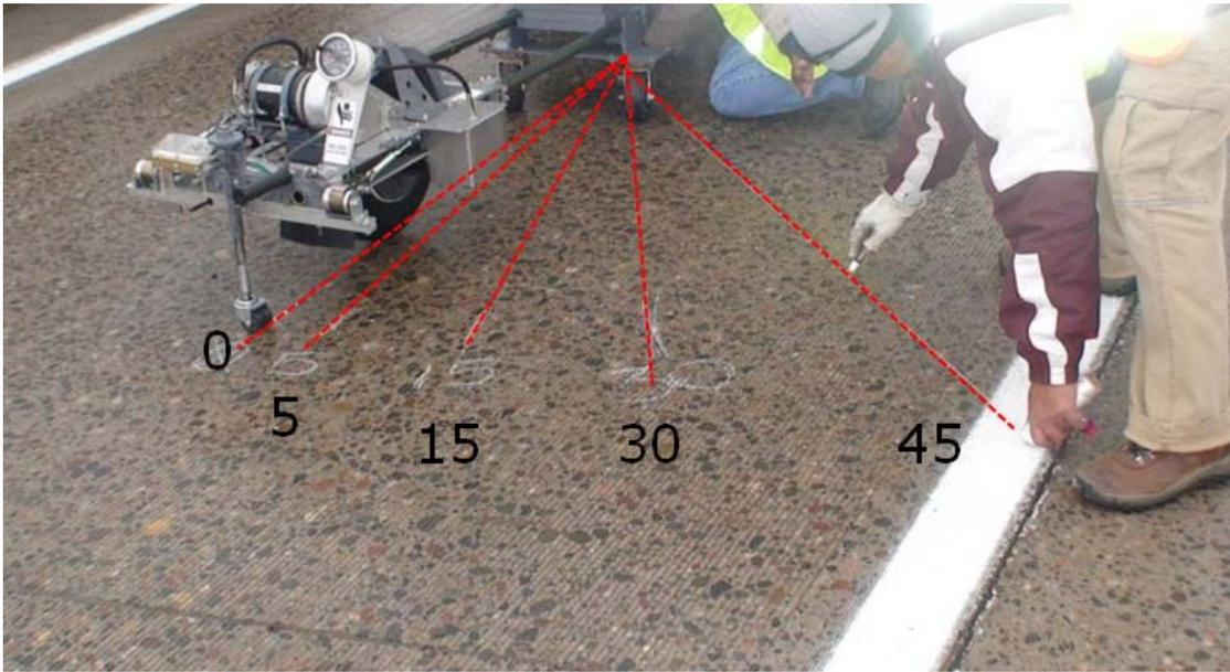
Figure 15. Photo of California CT-342 test device and selected angles of testing.
