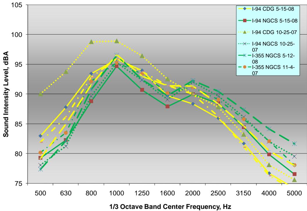
Figure 11. 1/3-octave spectra plots for I-94 and I-355 CDG and NGCS test sections.
