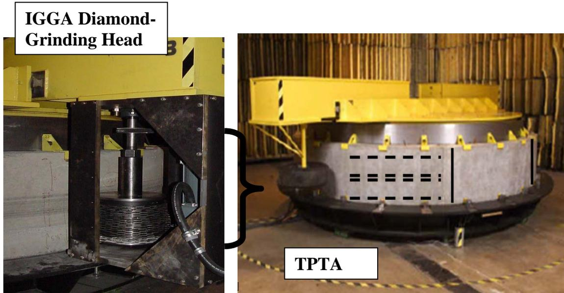
Figure 1. IGGA diamond-grinding head and Purdue Tire Pavement Test Apparatus (TPTA).
