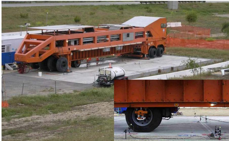
**Figure 4. Accelerated pavement testing using HVS on the precast panels for the I-15 Ontario project.**
