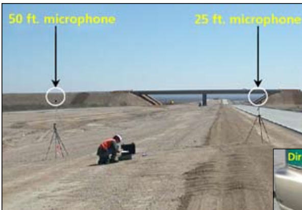
Individual passby testing with reference vehicle
