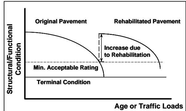
Figure 2. Increase in pavement life due to rehabilitation
