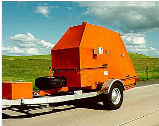
A falling weight deflectometer can identify the extent of delamination, or de-bonding, between pavement layers.
