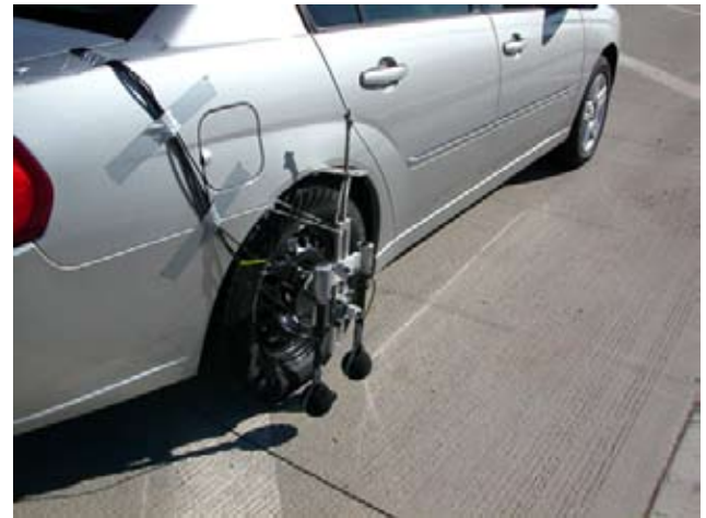
Typical On Board Sound Intensity (OBSI) dual probe installation.
