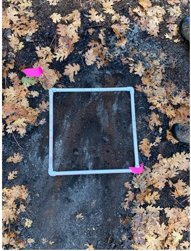
An example of a pile in which 90-95% of the white ash was scraped away from the half-meter square, seen in white, using a fire tool called a McLeod.
