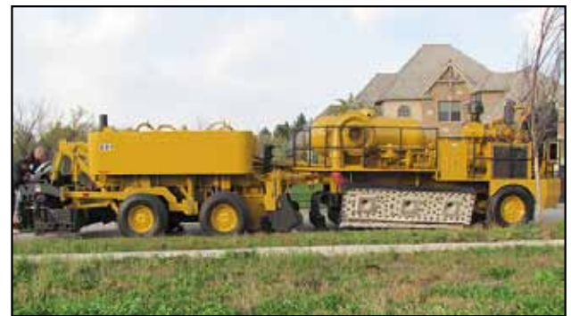
Figure 2. Reheater unit for 1-step HIR
