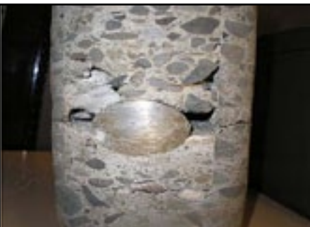
(e) Poor consolidation
