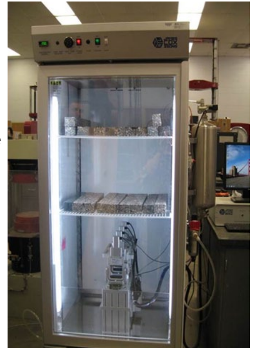
Figure 4. Finished beams and Coppers 4 pt. fatigue test equipment
