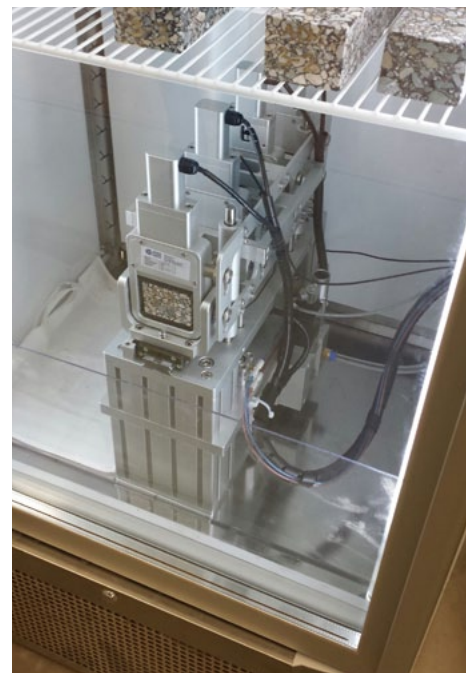
Figure 1. 4 Point Beam Fatigue Testing Apparatus
