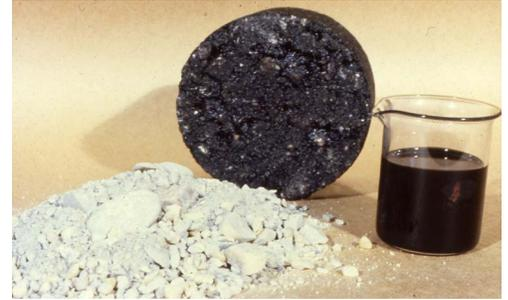
Asphalt Binder and Aggregates = Hot Mix Asphalt
