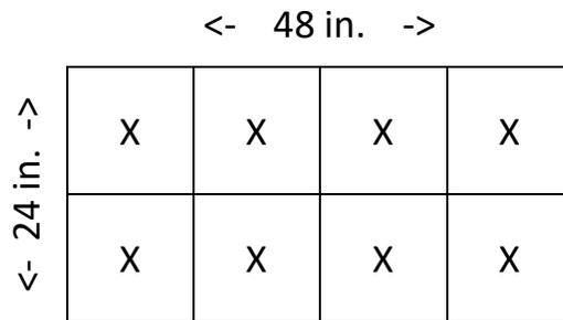
6. Record each reading on the Fume Hood Inspection spreadsheet. Average face velocities and record.
