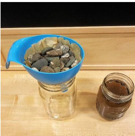
Our filter (left) was made from sand, gravel, and small rocks.
