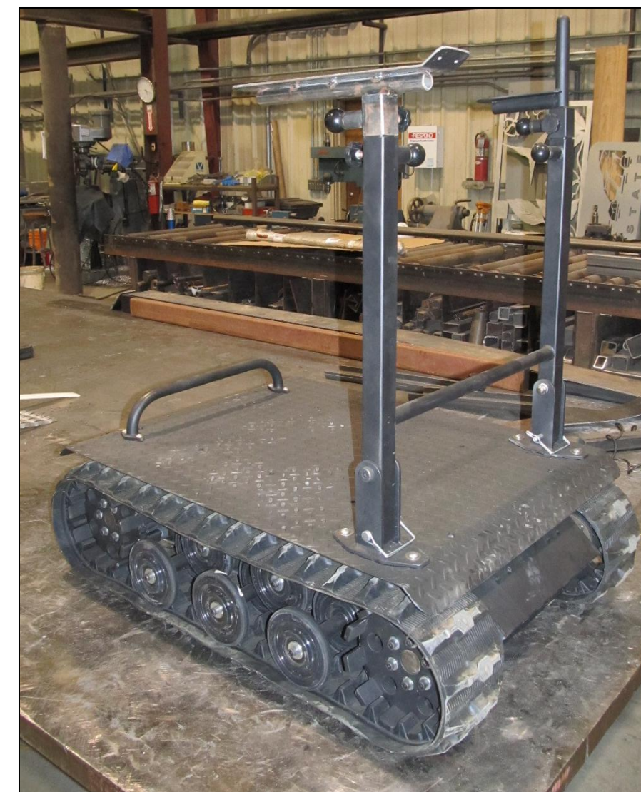
BTMV Device With Handle Bars Folded Down for Easy Transportation
