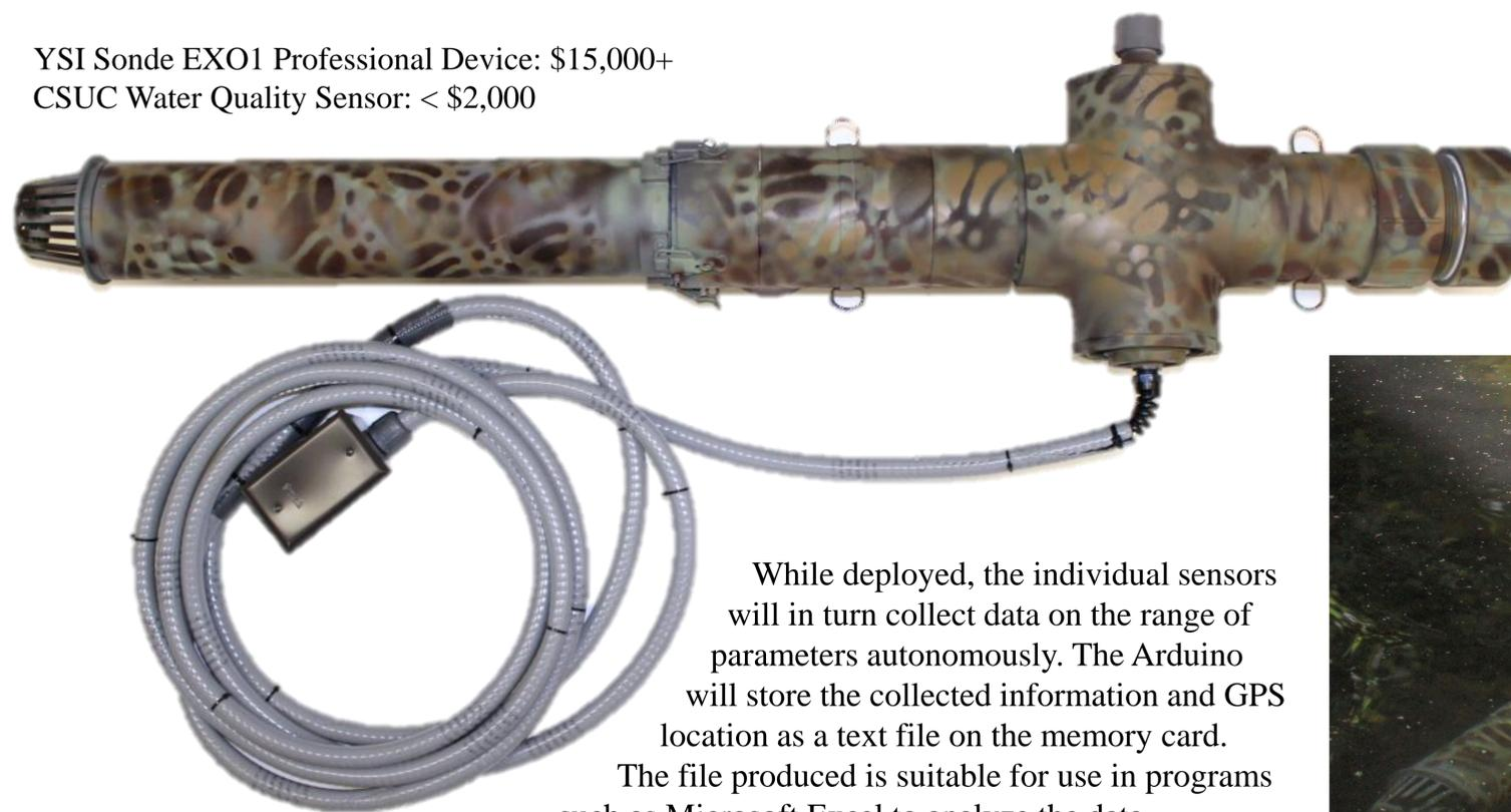
While deployed, the individual sensors will in turn collect data on the range of parameters autonomously. The Arduino will store the collected information and GPS location as a text file on the memory card. The file produced is suitable for use in programs such as Microsoft Excel to analyze the data.
