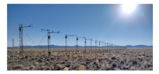
**Above:** A linear array of 50 ultrasonic anemometers, spaced 5 meters apart and located 4 m above the ground, was used to measure turbulence structure over the flat, dry, and uniform ground near Tonopah, Nevada, during the summer of 2023. The measurements will be used to test a recent theoretical development.
